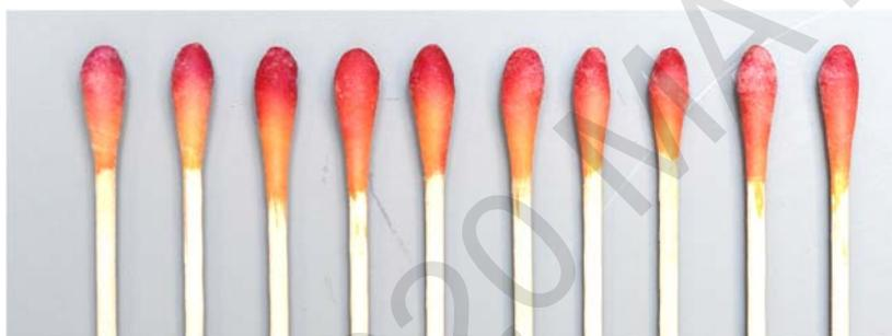
**Figure 2.** Reproducibility of the chromium-6 test at 0,5 µg chromium-6.
